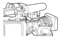
4 Connect the microphone connecting cable to the MIC IN jack.
